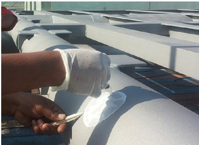
Figure 11. Attachment of paper to substrate.
