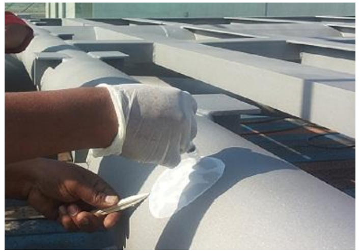
Figure 11. Attachment of paper to substrate.
