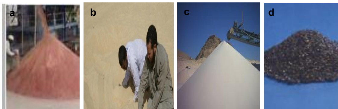
Figure 1. Samples from naturally occurring ores showing: (a) garnet abrasive; (b) sand; (c) white sand; and (d) ilmenite.
